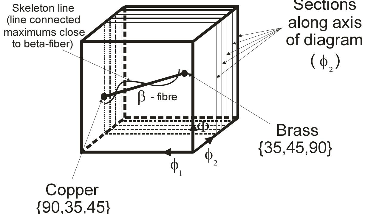
Below you can see skeleton lines diagram for  $\beta$ -fibre with 'Fill' option on:
