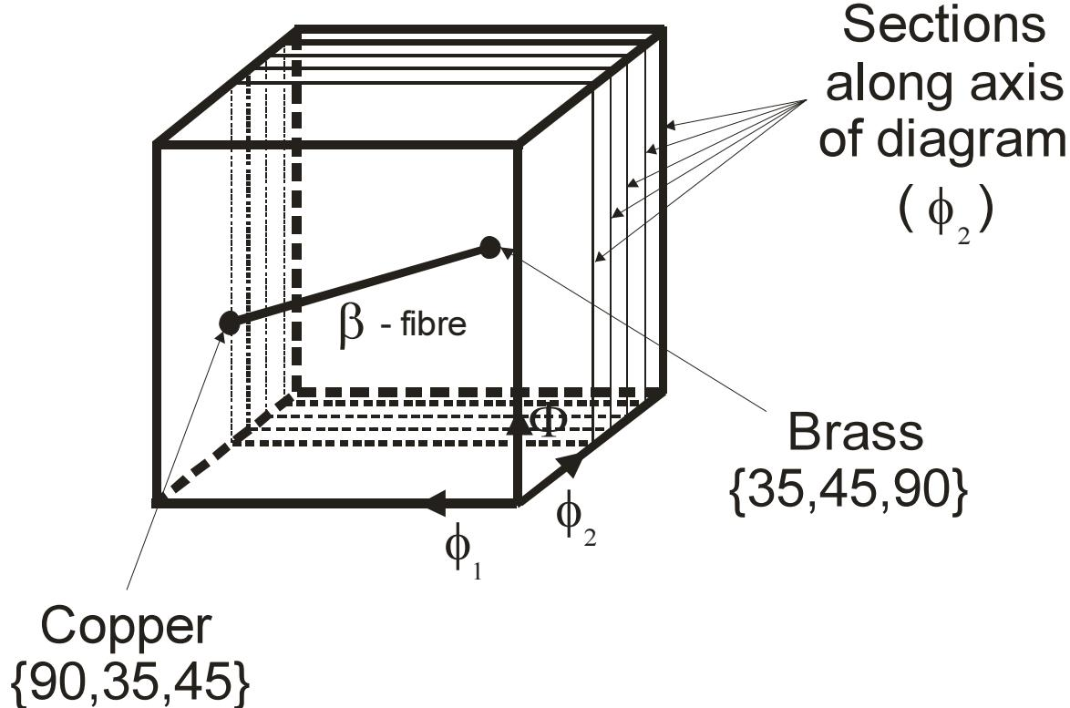
Example of section along axis of diagram
